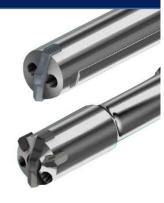
Fusible high-strength carbide Special geometry reducing to ultra-fine powder dust.
