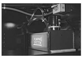
Coolant system lubricates parts and flushes away chips. When optional portable cabinet is purchased, pump comes mounted inside cabinet.
