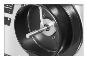
Interchangeable race assemblies size, finish, and work-harden parts in seconds; through-feed or up to a stop-and release.
