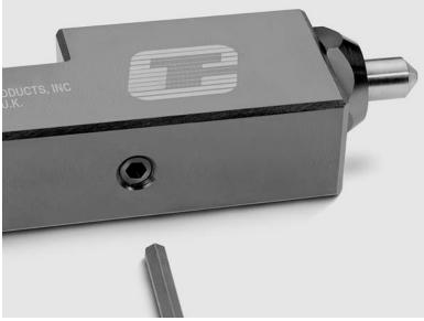
Diamond Burnishing Tools are adjustable for optimum burnishing pressure. For the DB-1 and DB-2 models, the adjustment screw is located in the end of the tool. For models DB-3 and DB-4, the adjustment screw is located on the side of the tool.
