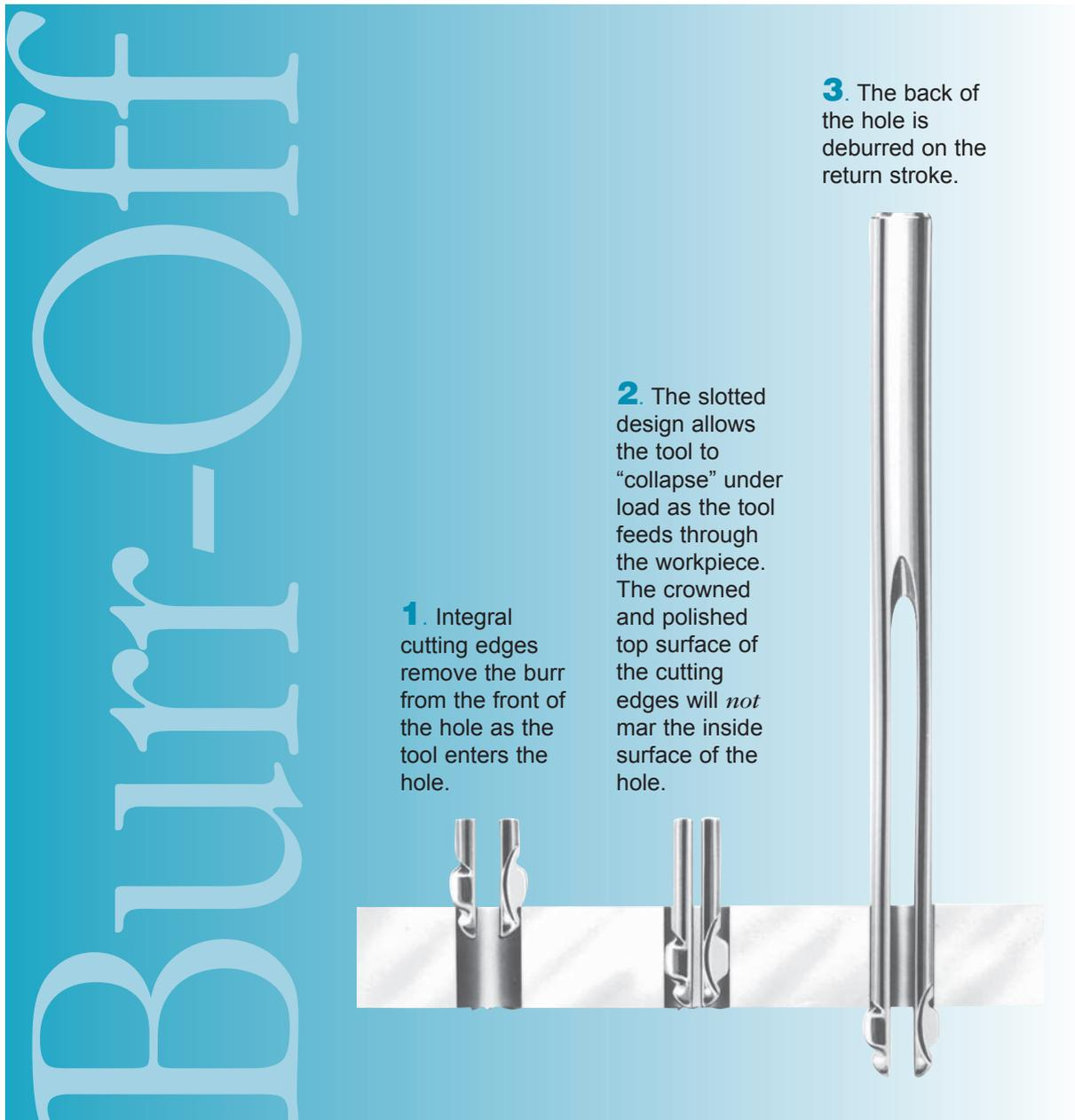
*The BURR-OFF® operates on the same basic principle as the BURRAWAY®, but is designed for high-production, automated deburring operations. The open-slot design of the “clothespin tool” allows chips to clear easily, which makes the tool ideal for automatic equipment and multi-spindle machines.*
