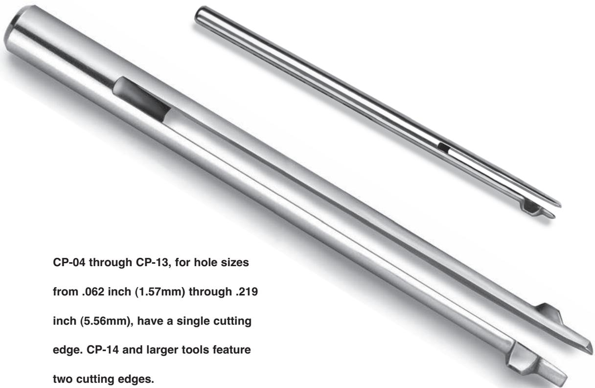
**CP-04 through CP-13, for hole sizes from .062 inch (1.57mm) through .219 inch (5.56mm), have a single cutting edge. CP-14 and larger tools feature two cutting edges.**
